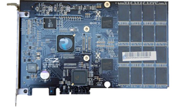
An OCZ RevoDrive SSD, a full-height x4 PCI Express card
