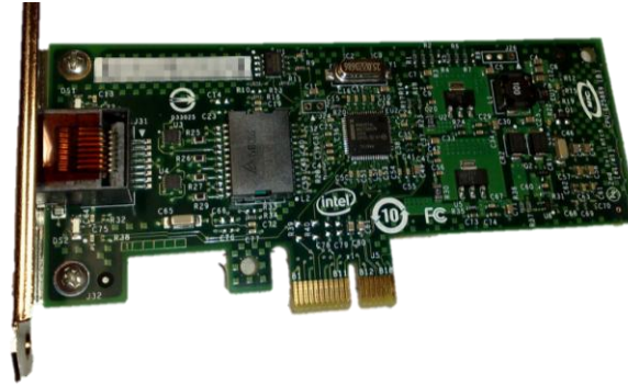
Intel 82574L Gigabit Ethernet NIC, a PCI Express x1 card
